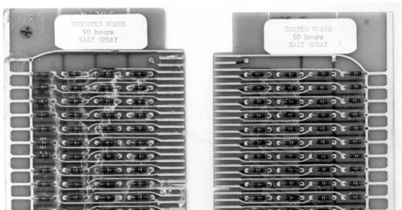
Figure 5.4. Effects of 50 hr salt spray on uncoated circuit board (left) and coated board (right).
