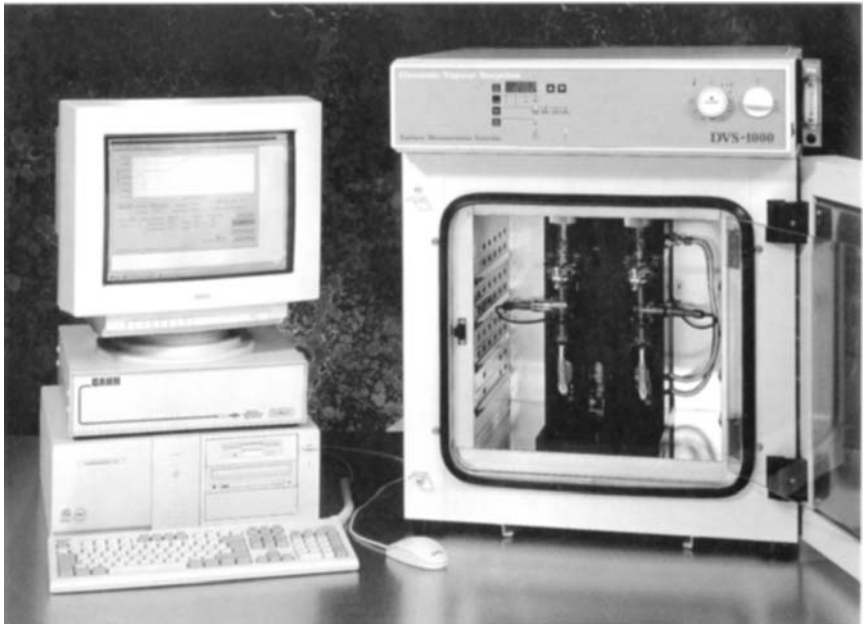
Figure 6.5. Dynamic vapor sorption analyzer. (Courtesy Surface Measurement Systems Ltd.)
