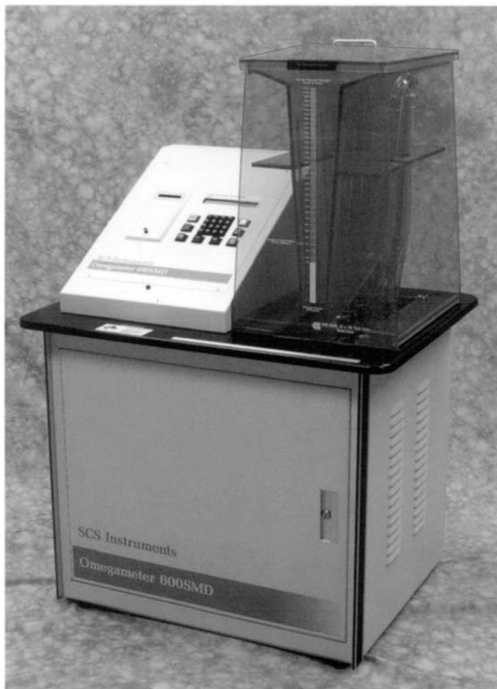
Figure 5.10. Omegameter® for testing cleanliness of electronic parts prior to coating. (Courtesy Specialty Coating Systems, a Cookson Co.)
