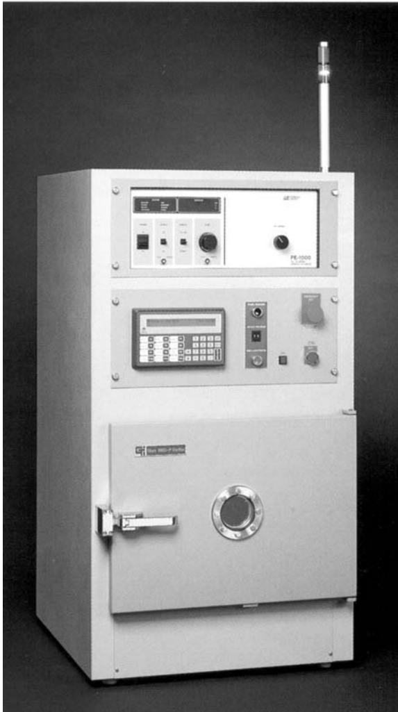
Figure 3.7. Plasma cleaner. (Courtesy Glen Technologies, Div. of Yield Engineering Systems.)
