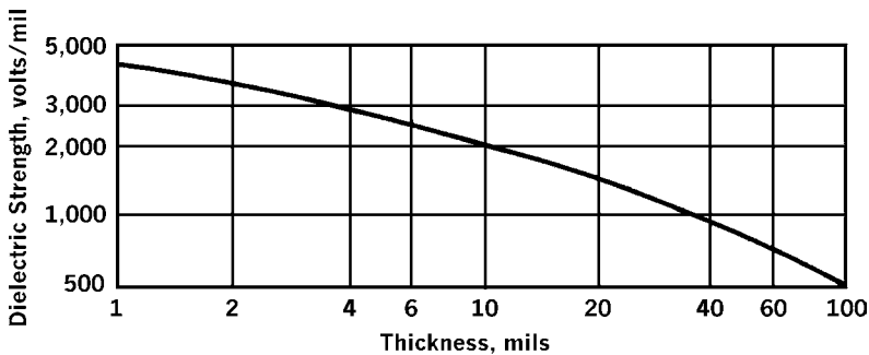
Figure 1.16. Effect of coating thickness on dielectric strength for Teflon TFE.
